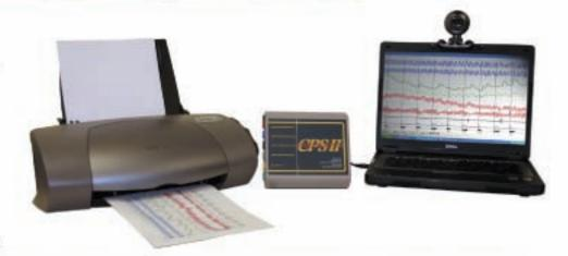
in 1968; the modular design in 1977; the CLC push-button re-centering in 1980; the Computer Assisted Polygraph in 1986; and the Computerized Polygraph System (CPS I) in 1990. In 2004, the CPS II was introduced, with newly designed hardware that eliminated the need for an external power supply and provides up to eight signal channels. Stoelting's intelligent design made CPS II what it is today, and its evolution helps meet your needs for the future.
