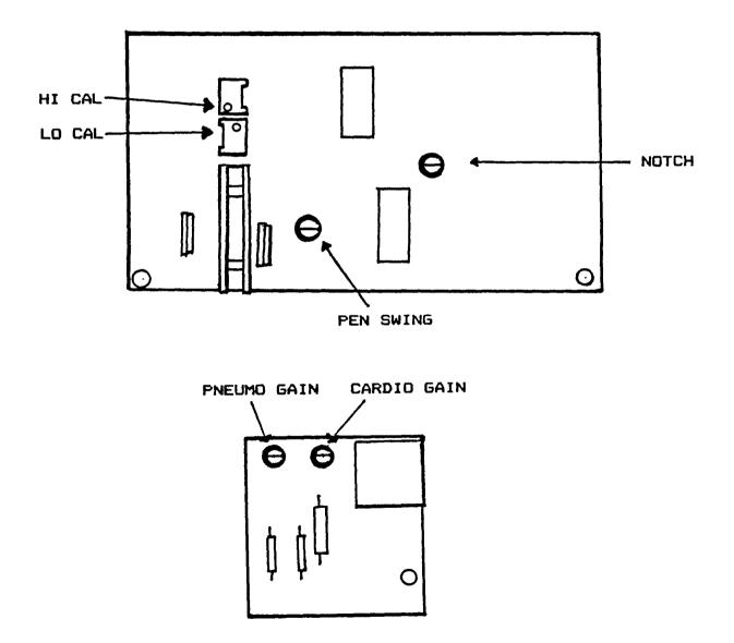
Note: If the trace is not as high in amplitude as it should be, and/or looks flat topped, the LO CAL trimpot should be adjusted to increase the Pneumo range, and/or eliminate the flat top.
