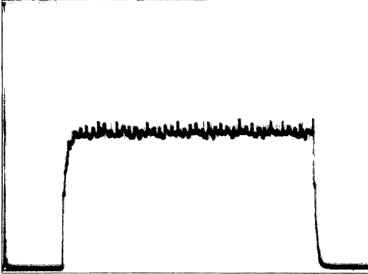
Figure 7. CVSA output when the input is an 8 millivolt peak-to-peak 1000 Hz sine wave (stressed response).
